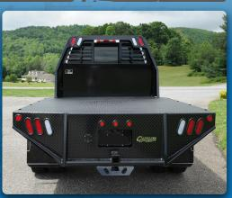
Steel is known for its brute strength and high payload capacity, it is made for your toughest jobs. Our all steel bed is made of 3/16" steel tread plate and is mounted on our heavy duty steel sub-frame, giving you a truck bed that exceeds industry standards.
